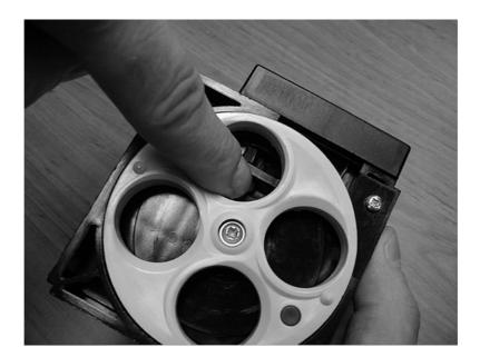
Insert a flat screwdriver as shown between the disc bed and gearbox cover and gently lift the gearbox cover.
